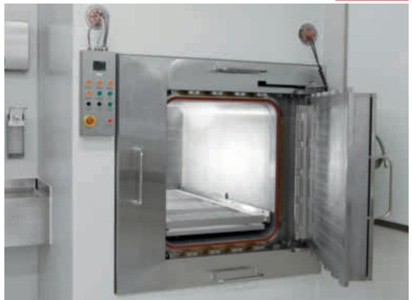
Double door chamber forms a barrier between hot and cold zones
